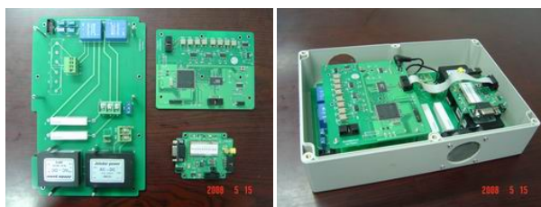
Fig. 12. Implementation of the sensing, processing and communication unit
